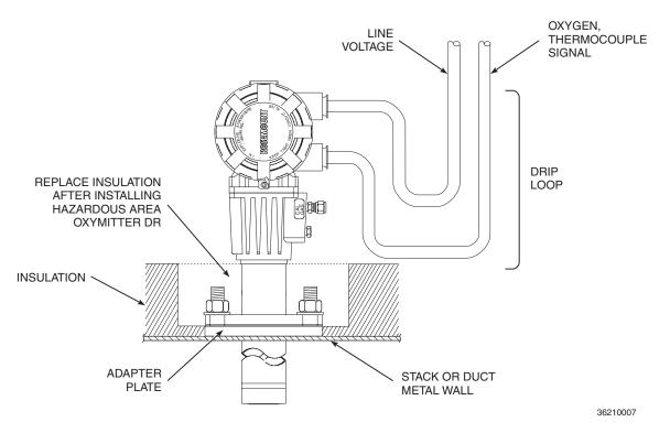
Figure 2-6. Installation with Drip Loop and Insulation Removal
